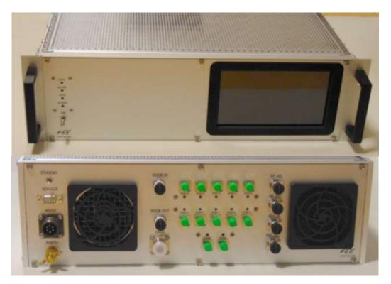
A front-panel touch-screen display allows ports configuration and internal signals visualization. There are options for high stability frequency additional internal reference. Power supply is 48VDC/50W, with dual input for redundancy.
