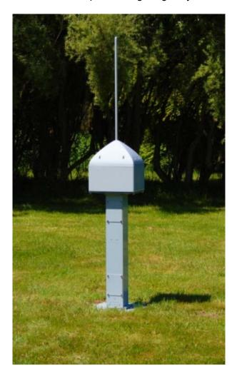
The picture shows a prototype antenna, its height is about 2.5 meters. This fully-integrated 2-30 MHz receive antenna includes integrated synchronous channelizing receiver and auto-calibration. Two GPS antenna (below radome) allow automatic relative positioning in the centimetric range when used in array, easing installation procedure. Calculations for relative positioning are done by the array controller remote computer from all antennas' preprocessed GNSS data.
