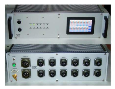
Each port is electronically protected, filtered, with its own power and energy meters, and can be powered on or off from front panel or remote control (Telnet on ethernet fiber). For a full-rated use, an 1.5 kW (minimum) 48..60VDC external power source is required, a second one can be connected for redundancy.
