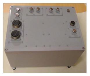
The receiver's architecture includes 2x 50-ohm Analog Front-Ends (AFE) modules feeding a 2-input digitization board which includes 2x 10G SFP+ ethernet links and 2x SyncNet ports, associated with a DSP daughter board.
